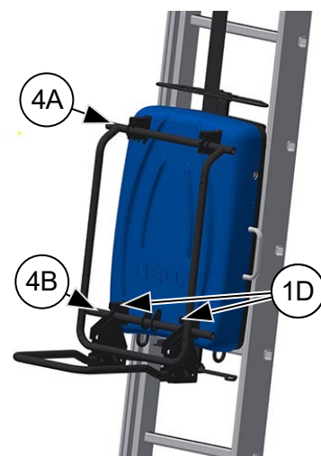
Afb. 47: Lastplatform "Basic" monteren
